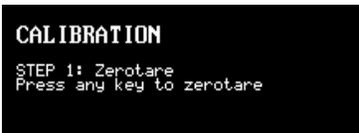
12. Press any key to initiate **Zerotare**. The LCD displays:
