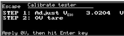
Short pins **5 and 6 together** on the **calibration fixture**. Then hit Enter (↵) key.
