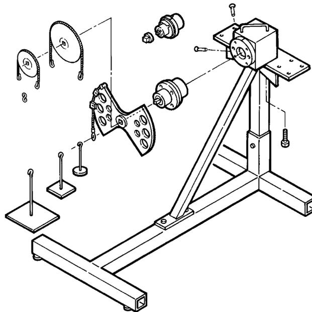
*Figure 5-1: Single Low Torque Transducer Mounting Detail*
