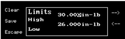
Sets up high torque limit preset. (-->) (F4) to go Down 1 line.
