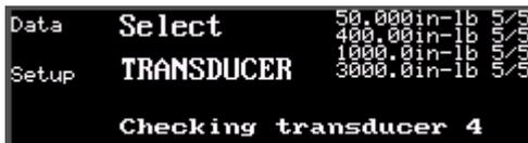
The user can either press F1 to display previously collected data (if any) or enter Setup Mode, F2. Any detected torque measurement will cause the *SURETEST* to enter Measurements mode where the following menu is displayed:
