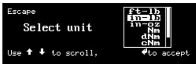
Selects the following Torque **units** on LCD display:
