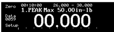
The *SURETEST* returns to the default menu from the measurements mode in the event there is no selection / input by the User for more than two minutes. This serves as a reminder for more (input) measurements.
