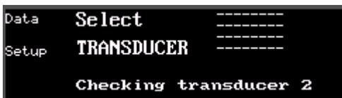
Select transducer by applied torque on it, LED will lit.
