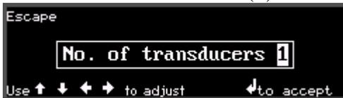
8. Using the Up (↑) or Down (↓) Cursor keys, enter "**1**" for a **single transducer**,
