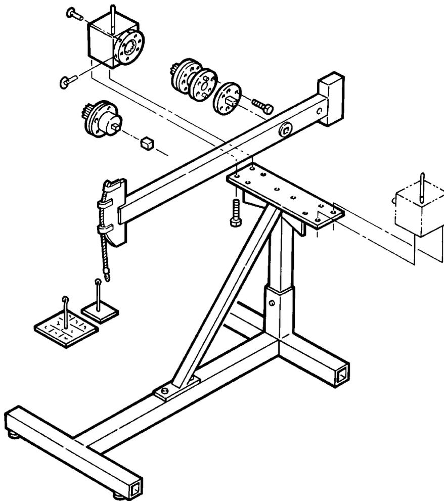
**Figure 5-2: Single High Torque Transducer Mounting Detail**
