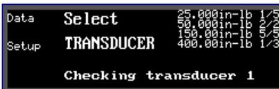
The user can either press F1 to display previously collected data (if any) or enter Setup Mode. Any detected torque measurement will cause the *SURETEST* to enter Measurements mode where the following menu is displayed:
