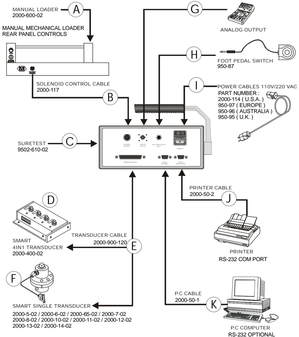
Figure 3-1: SURETEST Torque Tester/Calibrator/Loader Setup
