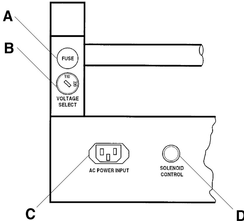
Figure 6-3: 2000-600-02 Manual Loader Rear Panel Controls
