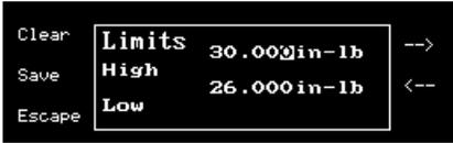
Sets up high torque limit preset. (->) to go Down 1 line.
