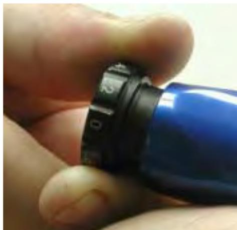
6. Place the 1/8" T-Shaped Hex in the back of the knob and Loosen the set screw. Pull the knob back and turn it until it is on the "0" increment of the knob is aligned with the 20% increment of the scale. Push the knob back to engage it and tighten the set screw. Recheck the reading.
