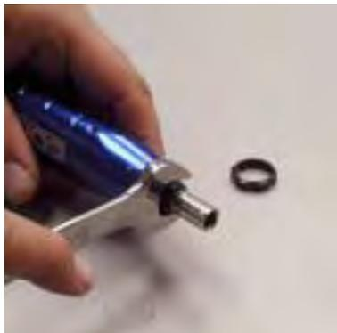
3. Replace the cone nut and tighten counterclockwise. Then tighten the cone nut to  $80 \pm 3$  IN.LB.
