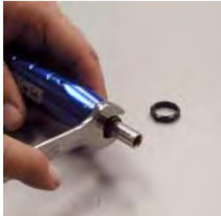
3. Remove the cam from the screwdriver.
