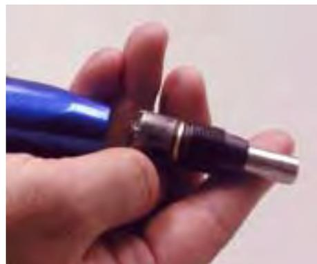
7. Perform a major calibration adjustment to bring the screwdriver within the accuracy limits or a minor adjustment could be used to bring the wrench within the accuracy limits.
