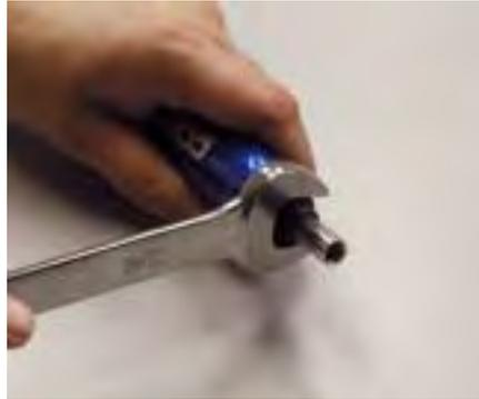
2. Turn the cone counterclockwise to remove from the cone from the screwdriver.
