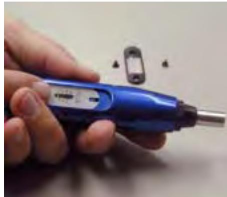
8. Place the Bezel over the scale and tighten the screws. Recheck the readings at 20, 60 and 100% of scale. If the screwdriver is calibrated torque the Bezel screws at  $3\pm.2$  IN.LB. Then the set screw to  $60\pm 2$  IN.LB. Place a new end plug on the end of the screwdriver.
