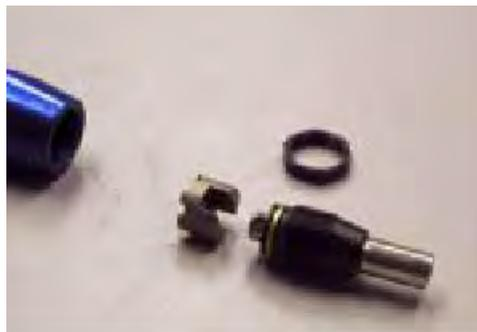
4. Inspect the secondary cam to assure that the spherical balls (2) are in place in the secondary cam. If they are not, grease lightly to hold them in the secondary cam.
