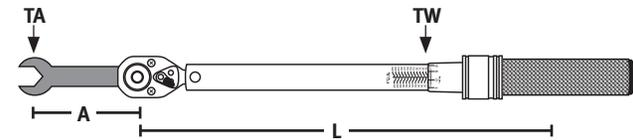
A number of variables can affect torque accuracy. These include the length of an adapter or extension, length of the wrench and variations in hand position on the wrench will affect the accuracy of the above calculation.
