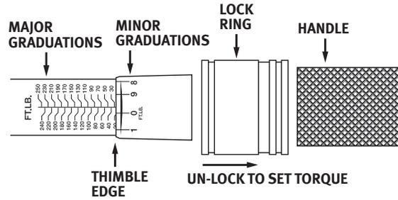
A. To unlock handle hold tube and pull lock ring back allowing handle to turn CW or CCW.
