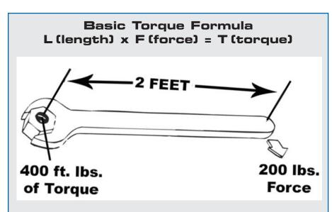
**Example:** A two foot lever at a right angle to the fastener with 200 pounds at the end will produce 400 foot/pounds of torque.
